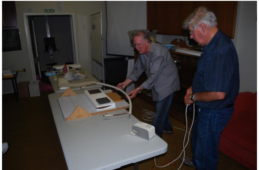
Flipped over and doing the bottom, note Terry managing the "power control, pull the plug out switch system". Barry uses an old ( very old) electric blanket controller for supplying power to the wire.
