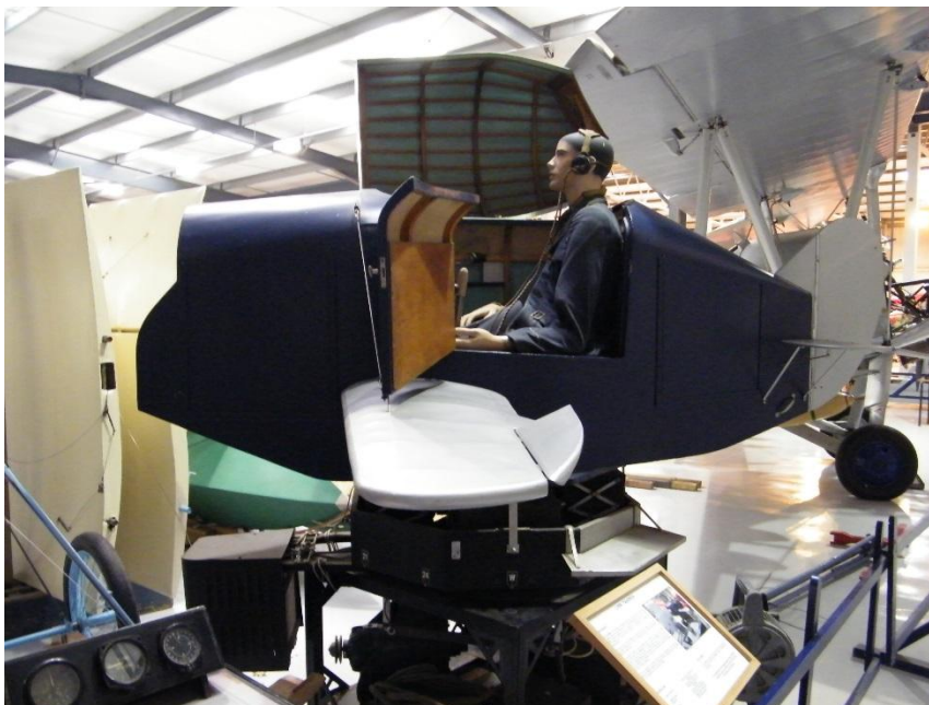
The LINK trainer. Who said Simulators are new. This was designed in the 30's, was used by the airforce thru to the 50's. Has been fully restored.
