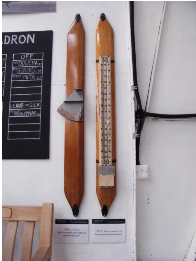
Instruments of yester year. On the left a strut mounted vane type airspeed indicator and on the right a strut mounted temperature thermometer.
