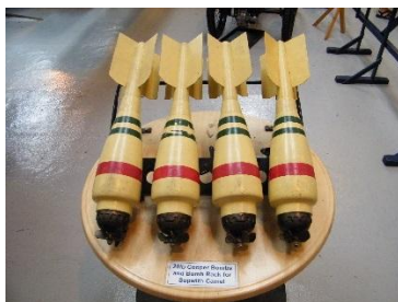
20lb Cooper bombs and bomb rack for the Sopwith Camel
