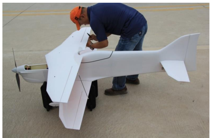
Composite fuselage, built-up wings and tail.
