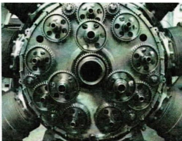
Drivers for actuating the combined and reciprocating action of the sleeve
