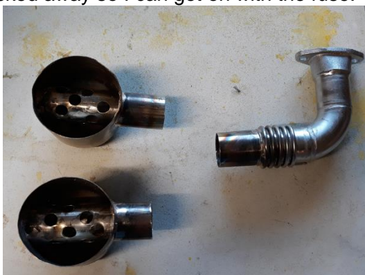
Shortened header. End caps with inputs for the bespoke muffler.
