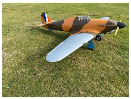
Scale; 1:4.5, Wingspan; 2710mm, Engine; DLE85 cc.
